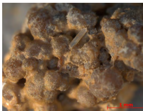
Fig. 1. Light green crust of turquoise from Sândomic, Romania (left) and yellowish brown hemispheres of aheylite-planerite from Parádfürdő, Hungary.
