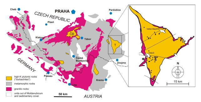
*Fig. 1.* Schematic geological map of the part of Moldanubian zone (left) and Třebíč Pluton (right) including pegmatite districts; dots = NYF pegmatite occurrences, star = Kracovice MIXED pegmatite. In part modified from NOVÁK et al. (2012).
