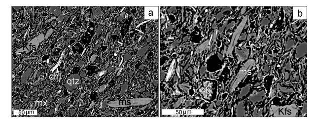
*Fig. 1.* BSE images of the ceramic body, with a fine network of partially melted clayey matrix (mx) embedding quartz (qtz), muscovite (ms), K-feldspar (Kfs), chlorite (chl) and carbonate (cb). The black parts are pores.
