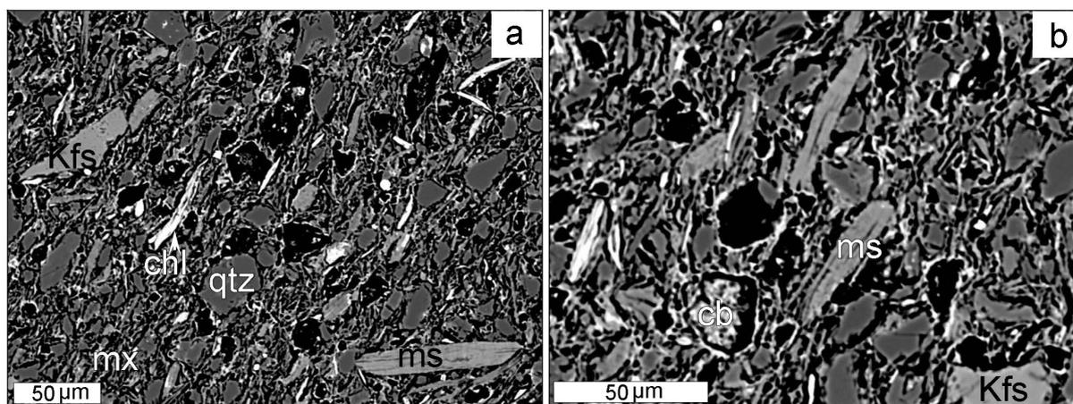
**Fig. 1.** BSE images of the ceramic body, with a fine network of partially melted clayey matrix (mx) embedding quartz (qtz), muscovite (ms), K-feldspar (Kfs), chlorite (chl) and carbonate (cb). The black parts are pores.
